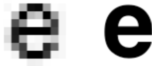
A 12-point Helvetica letter "e," enlarged 8 times. The letter on the left is from an Excel graph, showing the poor resolution. The letter on the right is from a drawing program (Inkscape).
